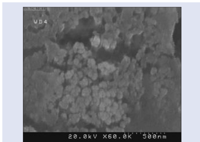
Figure 3: The field-emission scanning electron microscopy image of the green synthesized silver nanoparticles by reduction of aqueous Ag ions using Scrophularia striata flower extract under the optimized conditions
